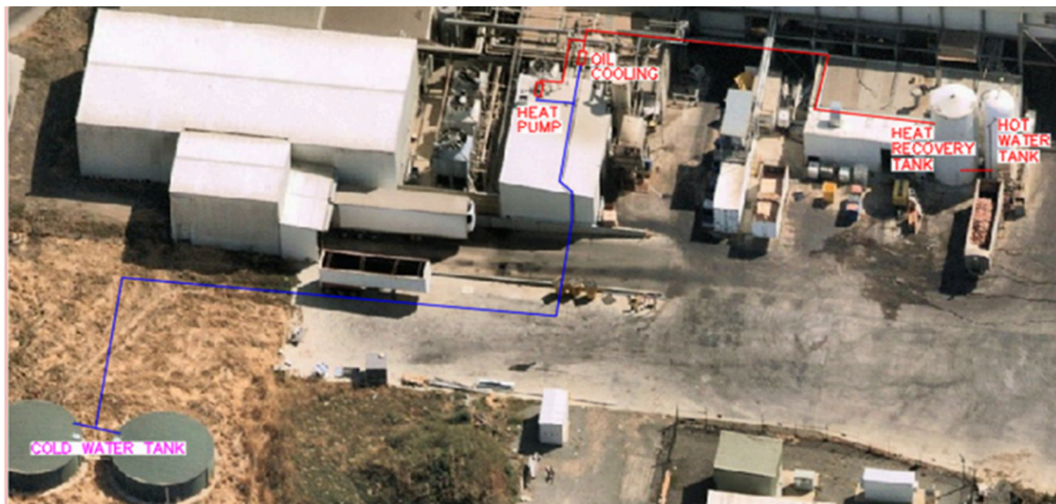
An aerial view and overlay diagram of the heat pump and heat recovery system set-up.
