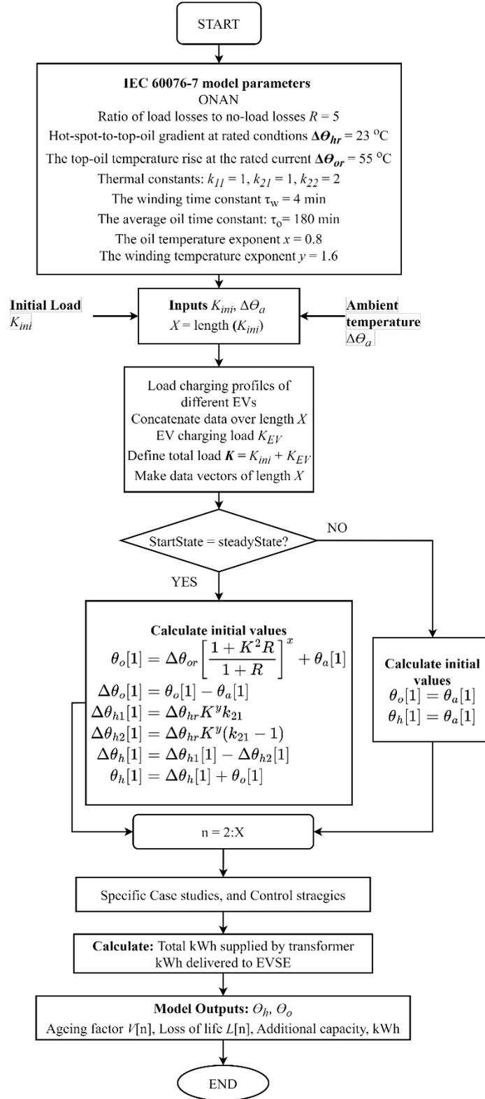
**Figure 5. Flowchart of the code developed around the thermal model described in IEC 60076-7. The code provides a suitable interface for users to set a range of model parameters and environmental variables. MATLAB code was utilised.**
