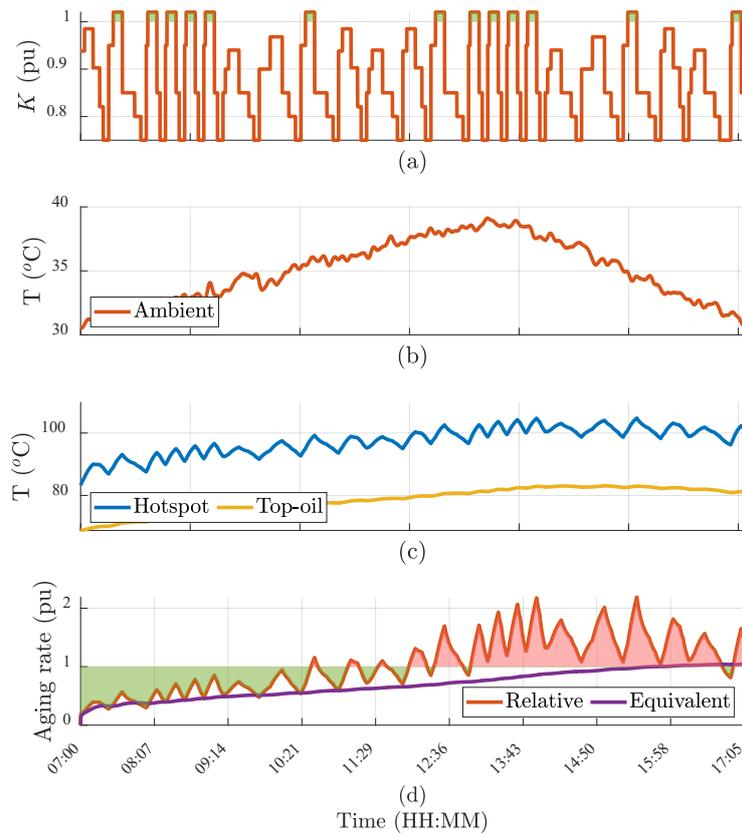
**Figure 8. EV charging impact on thermal performance of transformer using conventional Kraft paper, for non-EV load of 0.75 p.u., ambient temperature 30°C to 40°C with 5 min of idle time between charging sessions (a) Load factor, K (b) ambient temperature,  $\theta_a$  (c) hotspot temperature,  $\theta_h$  and top-oil temperature,  $\theta_o$  and (d) ageing rate.**
