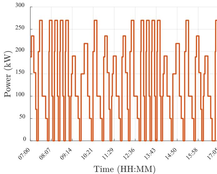
**Figure 7. The modelled stack of 23 charging session profiles of EVs.**
