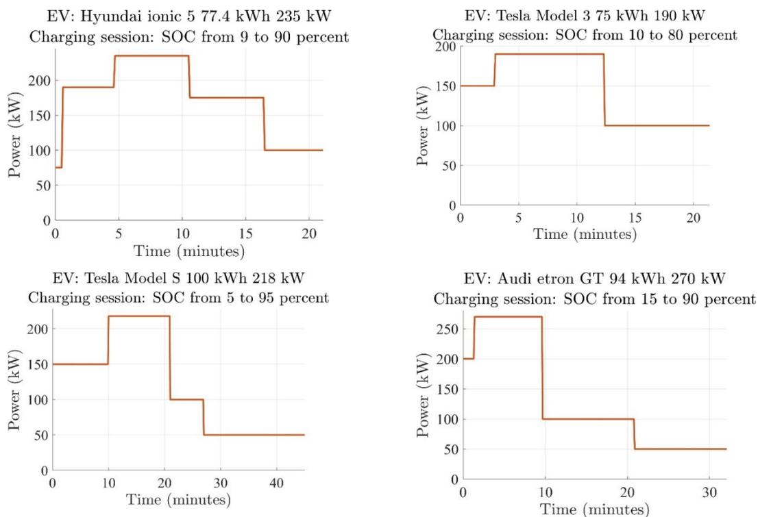
**Figure 6. Representative charging profiles of various EVs used in the study, with power averaged over different intervals to simplify simulation. Source: <https://www.fastnedcharging.com/en>**
