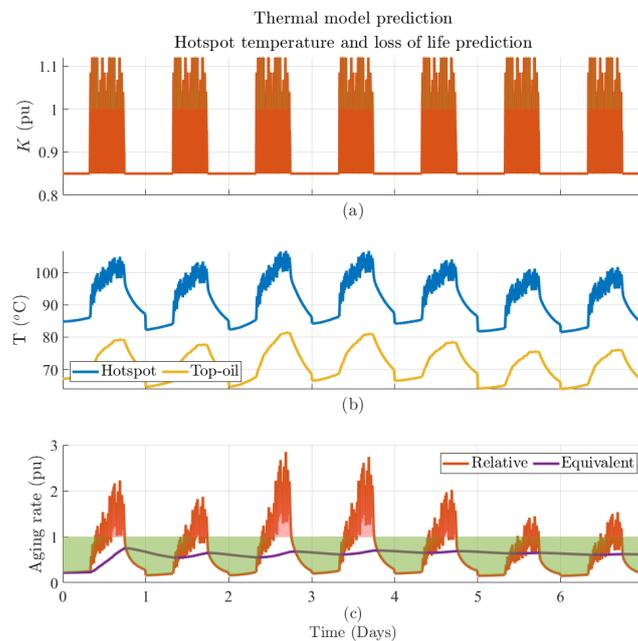
**Figure 9. Thermal performance and ageing analysis of a transformer over one week (January 1–7, 2023) in Byron Bay, NSW, based on representative EV charging profiles. A high non-EV utilisation of transformer at 85% and high EV congestion with new charging sessions starting within 5 minutes, from 8 AM to 6 PM.**
