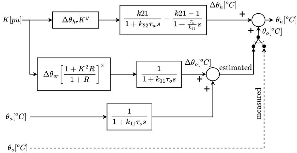
**Figure 4. Block diagram of the thermal model of a transformer provided in IEC 60076-7.**
