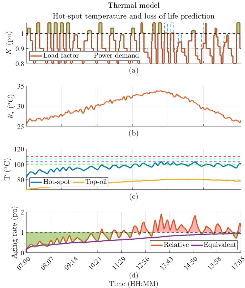
**Figure 10. Transformer thermal performance and ageing rate under multilevel hysteresis control, for Kraft paper insulation. Conditions: non-EV load 0.8 p.u. and ambient temperature range 25-35 °C.**
