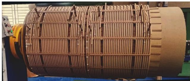
**Figure 2. Circular layer strap windings**
