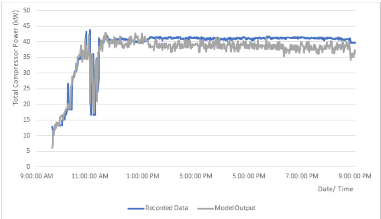
Figure 29 The measured and simulated total compressor power of the CO 2 refrigeration system in a subtropical aquarium for a 12 hour period on 06/12/2021
