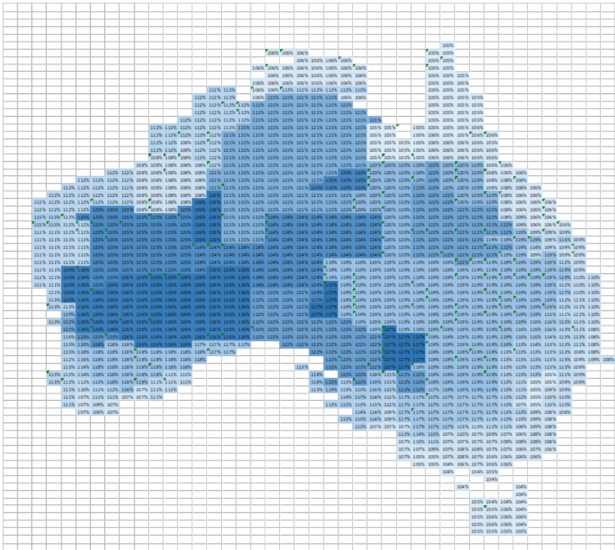
Figure 39 The ratio of the annual energy consumption of the refrigeration system for the abattoir case study for the adiabatic spray pre-cooling system vs the DP-CO 2 for different regions across Australia.
