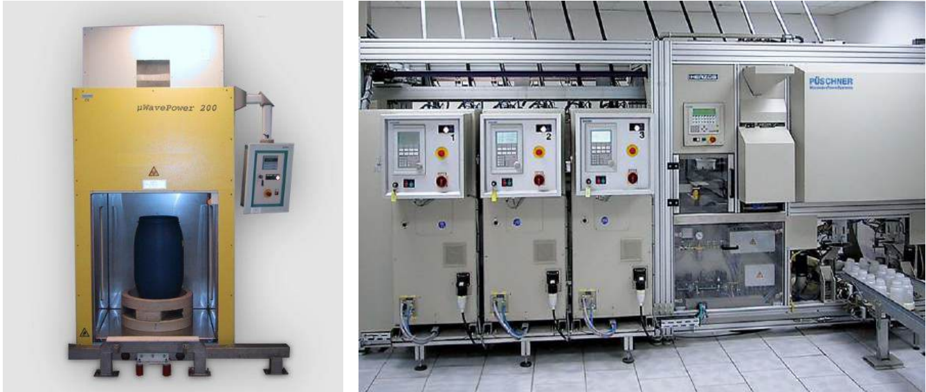
Figure 47. Small batch microwave oven from Pueschner (LHS) Continuous microwave system from Pueschner (RHS) [163, 164].
