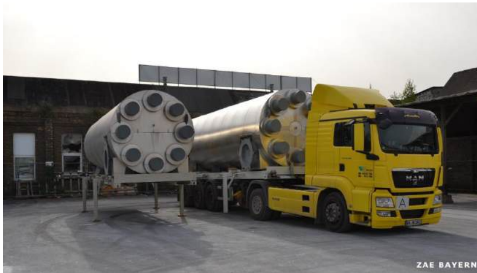
Figure 46. Mobile TES from waste heat source [158].
