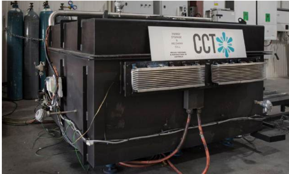
Figure 52. CCT Energy Storage's thermal battery [188].
