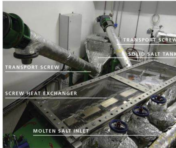
Figure 54. Overview of the storage test facility with screw heat exchanger with two shafts in front, two transport screws, and the tank for solid PCM in the back [194].
