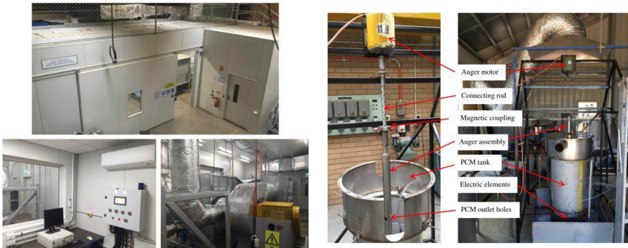
Figure 55. Left: High-temperature test facility; Right: auger melting rig at the University of South Australia [195].
