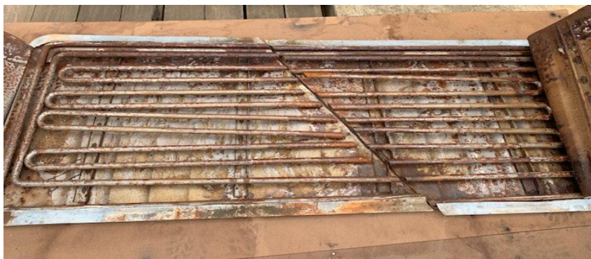
Figure 12. Interior of corroded eutectic plate.
