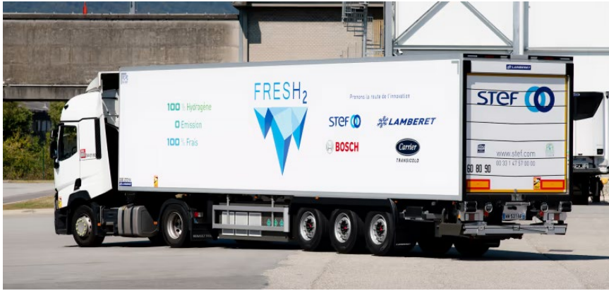
Figure 6. “Fresh 2 ” hydrogen fuel cell refrigerated transport (Carrier Transicold, 2021b).
